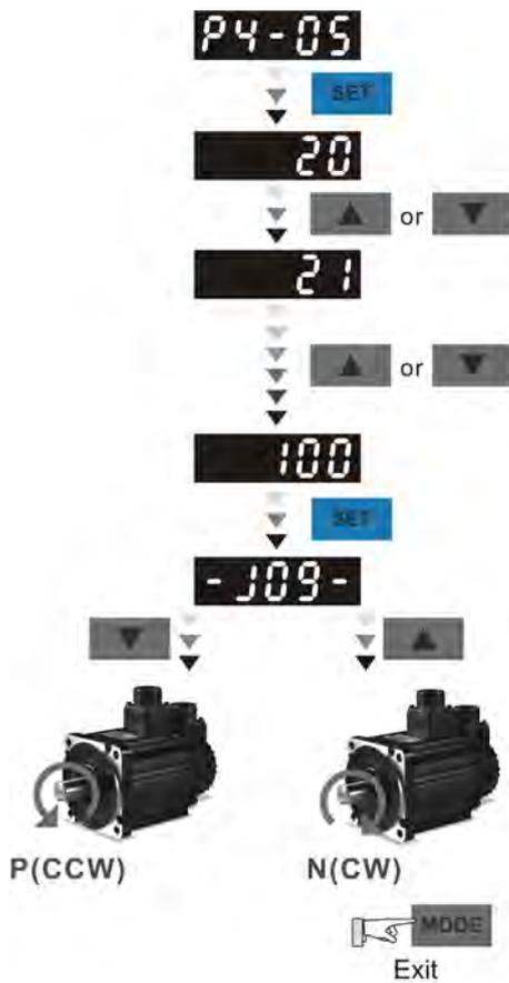
Pressing key and the servo motor will run in P(CCW) direction. After releasing UP key, the motor will stop running.
